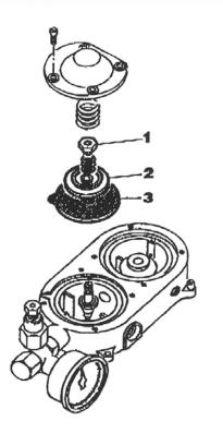
When reassembling the cap (# 2 fig. 62), be careful with the diaphragm centering ring (# 2 fig. 62). The nut (# 1 fig.62) must be screwed without force until it touches the ledge on the stem.
